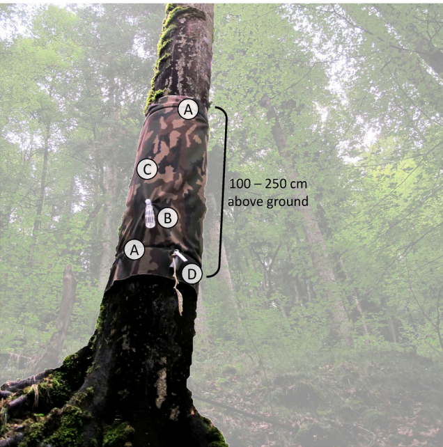
Fig. 2. Emergence eclector installed on a dead standing European beech tree to collect emerging saproxylic invertebrates. A = Metallic wire closing the extremities of the trap. B = Collecting device (plastic pipe + plastic bottle filled with 70% ethanol). C = Sampling surface. D = Temperature logger. Snags were sampled in the bole section from 100 cm to 250 cm from the ground.
